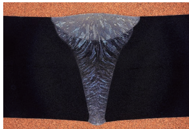
溶接の溶け込み
